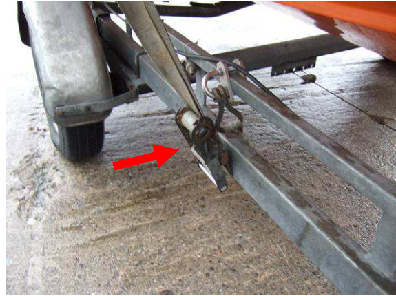
Note that the strap has to go under the trailer bar on the other side to stop the ratchet rubbing on the tube
