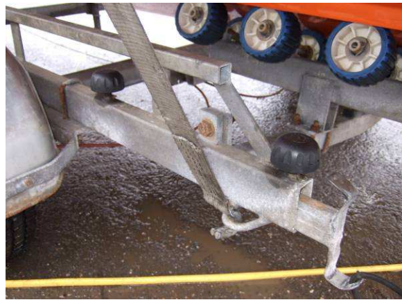
This is the rear of the trailer for the old boat – note there are two securing screws for the trailer bar on this boat.
