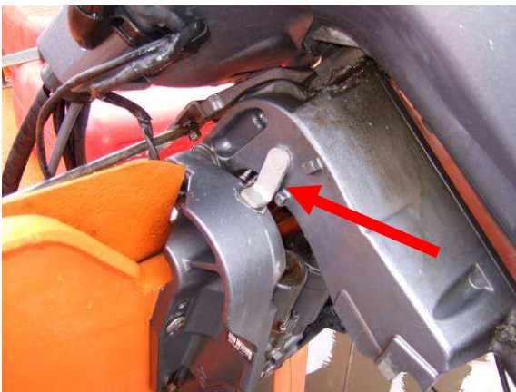
The boat engine needs to be raised a little before you pull it out of the boat shed to avoid it striking the ground by the door, and then raised fully. There is a “rest” that the engine should be lowered onto before trailing – see the shiny metal “L” in the middle of the picture of the engine.
